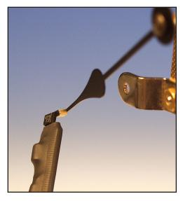
Stick the magnet to the tip of the minute hand so the red side faces away from the minute hand and towards the flat side of the sensor. Hold the magnetic sensor in a "third hand"
