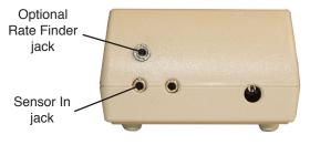
Plug the acoustic sensor into the jack labeled "Sensor In" at the top end of the
