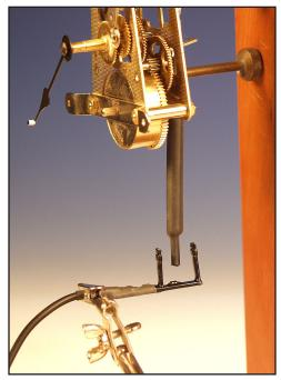
The optical sensor measuring a temporary, fast pendulum
